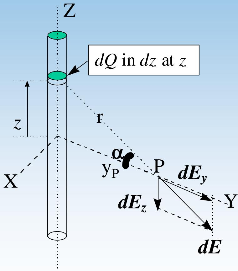
$z$ ,  $r$  and  $f(\alpha) \rightarrow$  write  $z$ ,  $r = f(\alpha)$  and integrate over  $\alpha$ .
